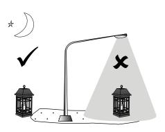
Do not position under bright light as this will prevent the light switching on at night.
