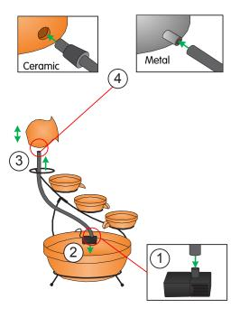
Attach tubing to pump and place in bowl. Pass tubing through top ring and fit to jug (use bung with ceramic or push straight on with metal jugs.)
