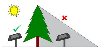
Position the solar panel to receive the maximum amount of direct sunlight.
