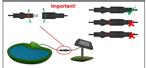
Ensure connection from solar panel to pump are water tight.
