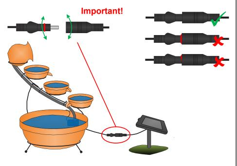
Ensure connection from solar panel to pump are water tight.
