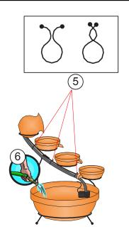
Use clips to hold tubing to frame and fill bowl with water.
