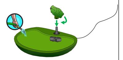
Insert pump with tube/bung assembly into the bowl. Position the pump so the tube protrudes through the hole in the bowl. Lower the spouting feature onto the tube. Ensure the bung seals, then lock the feature onto the bowl by turning slightly. Fill the bowl with water, ensure it is regularly topped off.
