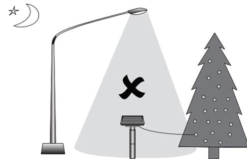
Do not position the solar panel under a light as this will prevent the light from switching on at night.
