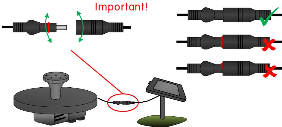
Ensure connection from solar panel to pump are water tight.
