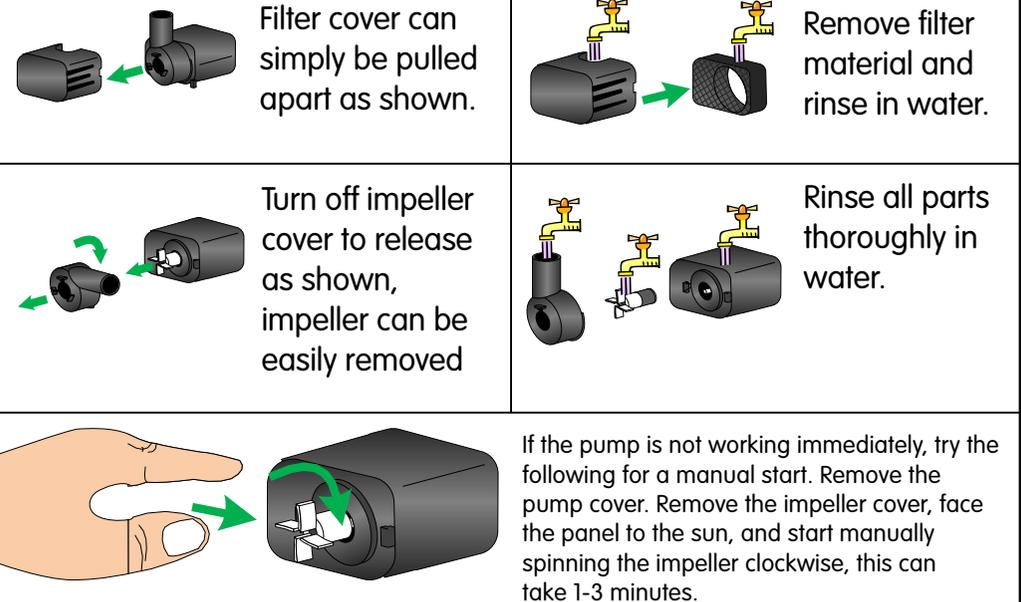
If the pump is not working immediately, try the following for a manual start. Remove the pump cover. Remove the impeller cover, face the panel to the sun, and start manually spinning the impeller clockwise, this can take 1-3 minutes.
