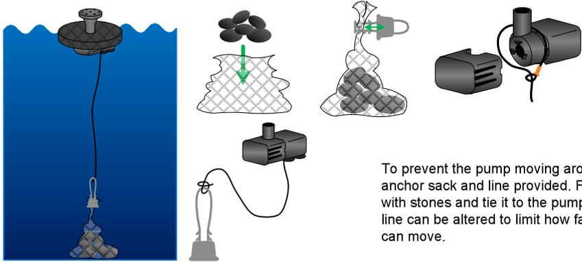
To prevent the pump moving around use the anchor sack and line provided. Fill the sack with stones and tie it to the pump, the length of line can be altered to limit how far the pump can move.
